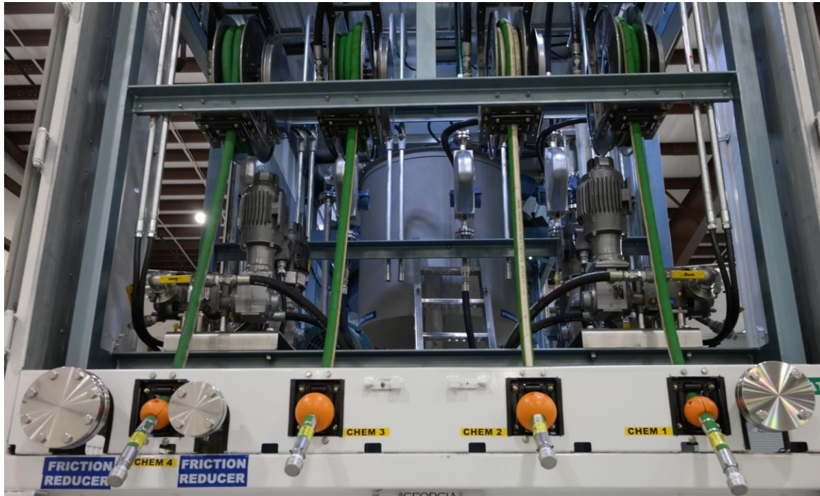
DISCHARGE POLYMER SOLUTION, MANIFOLD
