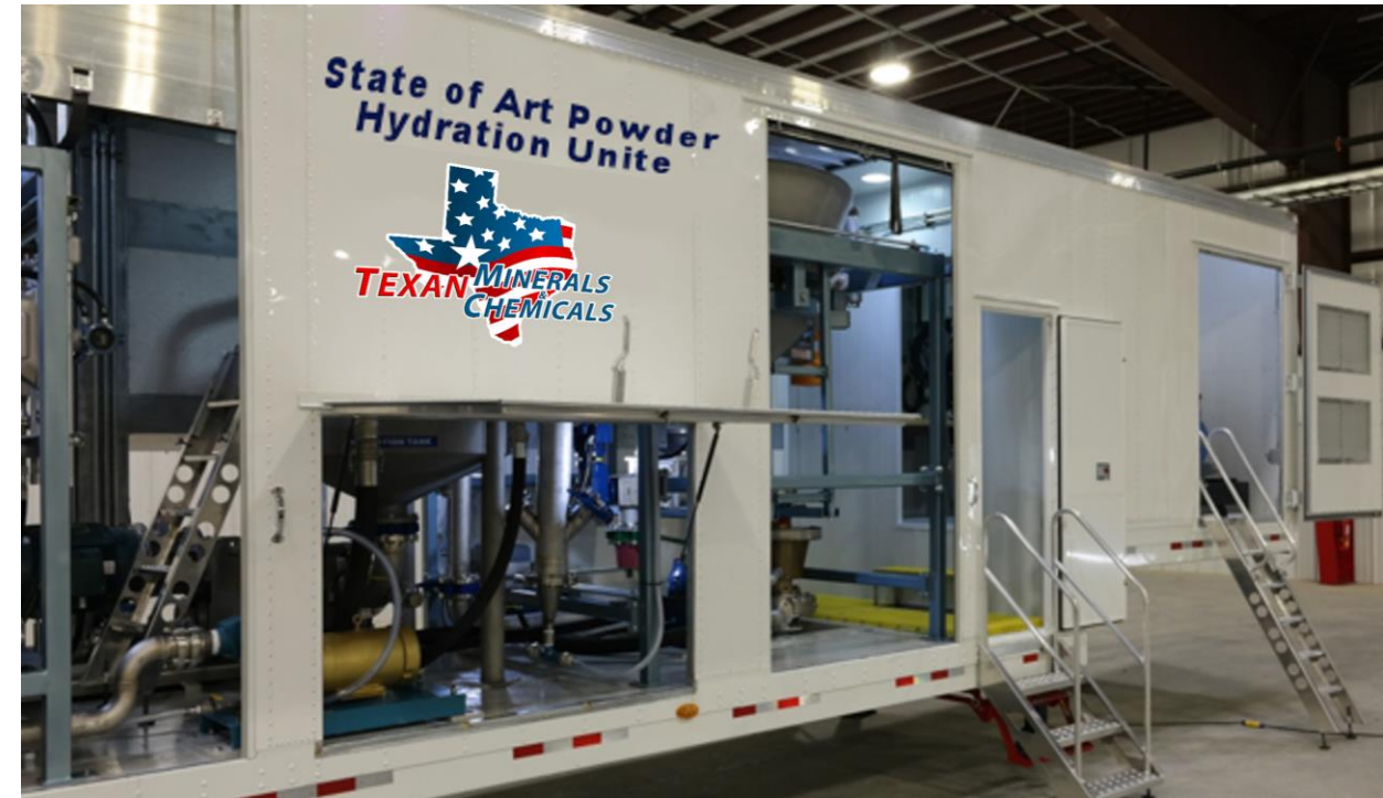
SUCTION PUMP → HOPPER & MIXERS → FRAC VAN INTEGRATION
